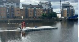
Modular pontoons cost effective, easily road transportable and built to size on site. To give a range of various sizes and rigged to suit clients needed. Can also be doubled up to increase deck load. Moonpools, Winches, scaffolding, Dive spreads, etc A great work platform.
